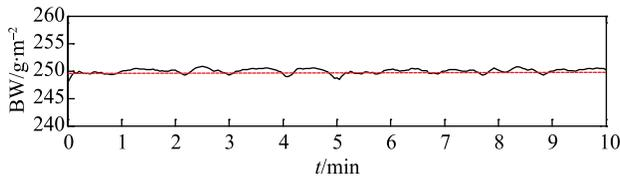
Fig.9 Curves of quantitative longitudinal change under stable condition
