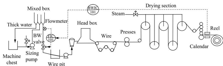
Fig.1 Schematic diagram of fourdrinier papermaking process
