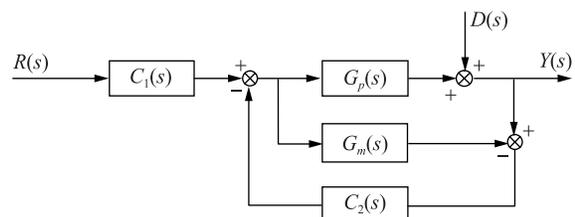
$C_1(s)$  is the set-point tracking controller;  $C_2(s)$  is the disturbance attenuation controller.
