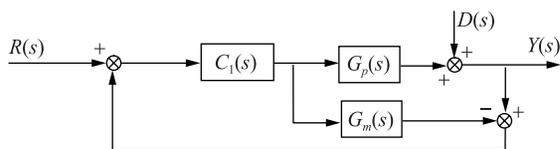
$Y(s)$  is the system output;  $R(s)$  is the set-point;  $D(s)$  is the load disturbance;  $G_p(s)$  is a stable process;  $G_m(s)$  denotes the mathematical model of  $G_p(s)$ ;  $C_1(s)$  is the primary controller of the IMC.
