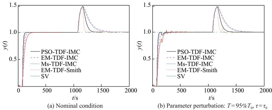
Fig.8 Simulation curve of paper basis weight control
