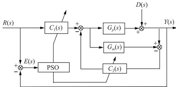
Fig.4 Control scheme of PSO-TDF-IMC
