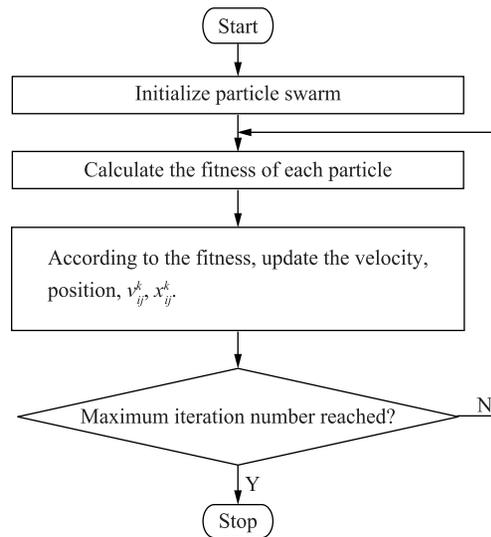
Fig.5 Flowchart of the PSO algorithm
